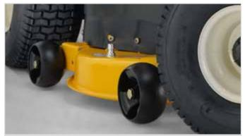
Anti-scalping deck wheels to prevent damages to the turf especially on tight turns.
