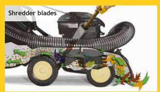
Internal shredder blades are reducing the volume of leafs and small twigs in a relation of up to 8:1. After vacuuming and shredding the material is automatically transferred into the felt catcher.
