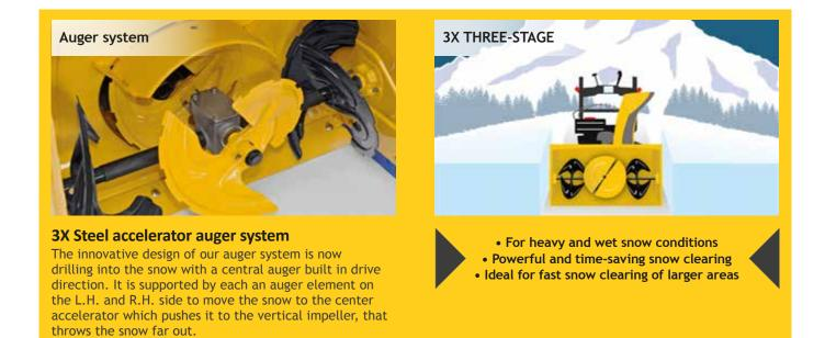
The revolutionary 3X-Series with 3-stage technology. At first stage two X-treme segments in the outer part of the auger housing are pushing the snow to the center, where at second stage a central X-treme segment drills through the snow and pushes it to the third stage, the impeller, which powerfully throws the snow through the chute channel far away into the desired direction.
