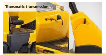
The Transmatic transmission allows shift-on-the-go speed control. Simply choose the driving direction, set the desired basic speed and start mowing. On the Cub Cadet ride-on mower CC 114 TA, you have the choice of 6 forward and 6 reverse speeds.
