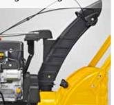
The discharge chute is exceedingly high and consists of plastic on the 2X Series. It is clog-resistant and assures an optimal discharge of the snow. Snow throwing direction and width can be adjusted conveniently from the dashboard.
