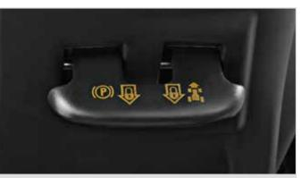
**Cruise control / Parking brake** With this lever you can set a cruise speed when driving and set the parking brake when the tractor is not in motion.
