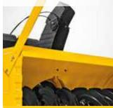
The drift cutters which are mounted on both sides of the auger housing, break deep snow banks away and thus allow the snow thrower to power through even the heaviest drifts. Better performance and easier working in extremely deep snow.
