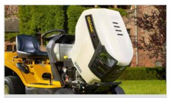
**Pivoting one-piece hood** The entire motor hood can be removed within seconds without the need for tools, for easy maintenance.
