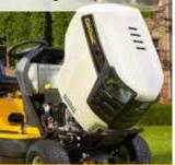
The entire motor hood can be removed within seconds without the need for tools, for easy maintenance.
