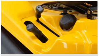
Cutting height adjustment & PTO clutch
