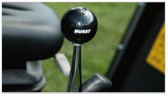
HURST shifter With the Hurst shifter you have the choice of forward/ neutral/reverse and low speed forward gears.
