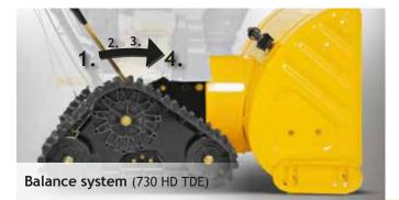
**1. Packed snow:** Bringing the lever in the "packed snow" position, the weight is shifted to the front end of the snow thrower and presses this on to the ground.
