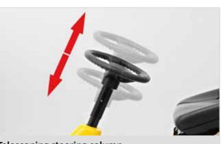
**Telescoping steering column** You can easily adjust the height of the steering column to suit to every operators height.
