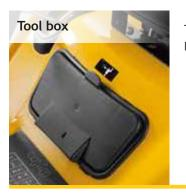
Tool box with integrated 12V power outlet.
