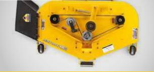
You have the choice of 3 different side discharge cutting deck sizes, 122 cm, 127 cm or 137 cm. The 122 cm deck is made of 2.8 mm thick fabricated steel and thus made for tougher jobs.
