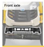
Pivoting steel or cast iron front axle. This keeps all four wheels on the ground also on uneven surface.
