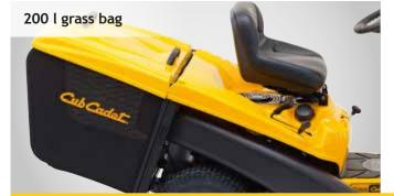
200 l grass bag with hard top (model CC 114 HA), grips and fill indicator. It can be dumped from the drivers seat.
