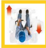
**Executing a zero-turn:** To execute a zero-turn, move one control lever forward while simultaneously moving the other control lever rearward.
