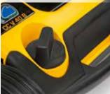
The working depth of the Cub Cadet scarifyer CC V 40 B can easily be changed centrally.
