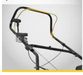
With the lever on the handle you can switch from transport to working position conveniently from behind the unit.
