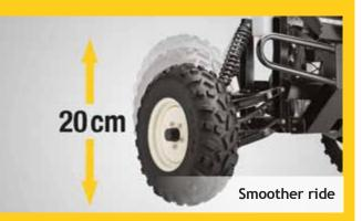
Independent dual A-arm suspension with coil-over shocks provides 20 cm of wheel travel for an unbelievably smooth ride. You'll cruise over the most challenging terrain for a remarkably comfortable experience that you only get from the best utility vehicles.
