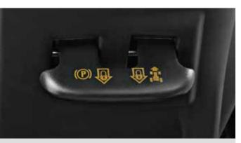
**Cruise control / Parking brake** With this lever you can set a cruise speed when driving and set the parking brake when the tractor is not in motion.
