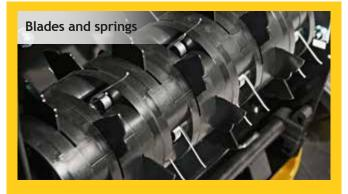
The CC V 40 B has 17 flail double blades and 16 double springs. This combination allows for two functions in one machine - for aerating and scarifying. If you would like to aerate the soil of your garden, use the higher position with a gentle touch of the blades and springs on the surface of the soil. If there is the need to scarify, use a deeper position of the blades and springs which allows having a more aggressive action on the surface.
