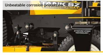
Provides twice the protection against unforgiving environmental conditions while ensuring even the most complex parts are thoroughly and evenly coated inside and out with an electronically-applied dual layer of eCoat and powder. Now that's a smart investment.
