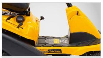
**Step-through frame** With soft rubber foot pads, for easy access and comfortable foot rest.
