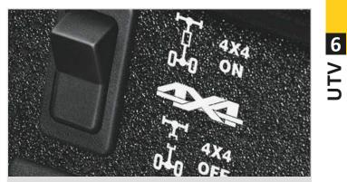
**Easy switch to 4 x 4** With a rocker switch in the dash, you can switch from 4 x 2 to 4 x 4 if required.
