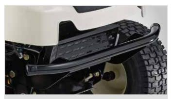
**Front bumper** Prevents your investment from damages and thanks to the Fast Attach<sup>™</sup> system you can replace the bumper with i.e. a dozer blade within minutes with no tools required.
