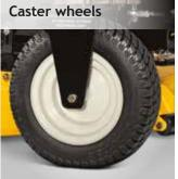
Controllable pneumatic front caster wheels which makes your TANK SZ versatile at is best.
