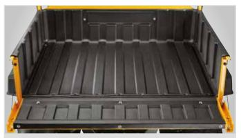
**Higher capacity** Large tiltable bed with optional electric cylinder. It fits a Euro palet and is suitable for tough jobs.
