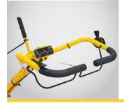
Single-hand operation lets you stand to the side and steer the tiller with one hand. Comfortable full bail handle with soft grips.
