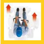
**Turning to the right:** To turn to the right, move the right drive control lever rearward of the left lever. The greater the distance between the two levers, the sharper the mower will turn.
