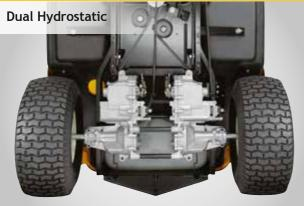
**Dual Hydrostatic transmission** The dual Hydrostatic transmission provides you with the highest manoeuvrability.
