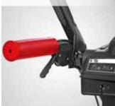
Keep your hands warm to finish the job in comfort! To activate the heated grips, iust move the switch found on the rear of the dash panel into the ON position. The handles stay warm and you can keep working through the coldest weather.
