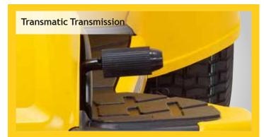
The Transmatic transmission allows shift-on-the-go speed control. Simply choose the driving direction, set the desired basic speed and start mowing. On the Cub Cadet ride-on mower CC 114 TA and CC 114 TD, you have the choice of 6 forward and 6 reverse speeds.
