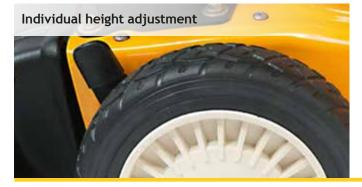
The vacuum nozzle distance to ground can be adjusted in 5 different heights from 16 to 104 mm with an adjustment lever at the front wheels. This enables you to adapt the vacuum to individual conditions. A higher adjustment can be of advantage on gravel walkways while a lower adjustment would be preferred on solid grounds.
