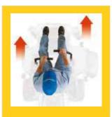
**Turning to the left:** To turn to the left, move the left drive control lever rearward of the right lever.
