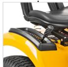
**MECHANICALLY SUPPORTED CUTTING HEIGHT ADJUSTMENT**
